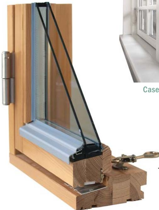
The bottom sash of the multi-layered deep-impregnated timber window is protected with an aluminium glazing bead. To reduce heat loss at the edge of the glass, we recommend using an insulated glazed unit that has SWS (plastic) spacers rather than the traditional metal.
