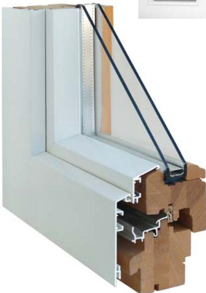
The wooden parts are made of three-layered deep-impregnated laminated timber. To reduce heat loss at the edge of the glass, we recommend using an insulated glazing that has SWS (plastic) spacers rather than the traditional metal.
