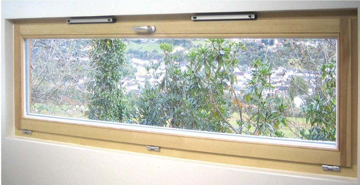
The "Aru 78 SOFTLINE IN" window with the angular profile sash and frame is an inward opening wooden window with a profile which is suitable for a modern energy saving building. The larger frame is designed to accommodate triple glazing. This increases insulation values enough for use in a so-called passive house.
