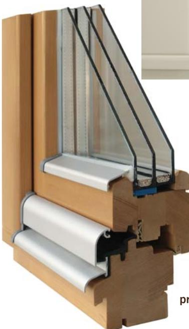
A three-layered deep-impregnated window, the bottom frame and sash are protected with aluminium glazing beads. There's an option of using concealed hinges and design Available with a choice of handles.
